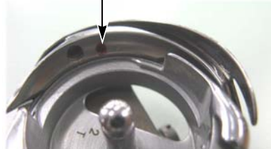
Lubrication hole (Red mark)
